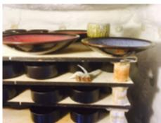
Gas fired kiln showing reduction-glazed work
