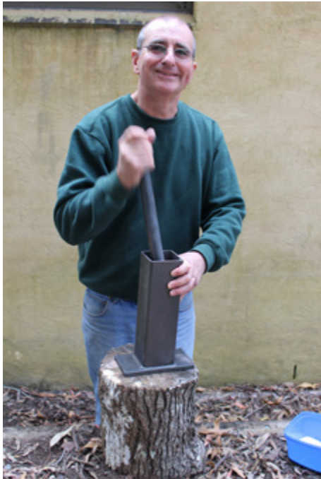
Rob Linigen, hand crushing bone ash for glazes.
